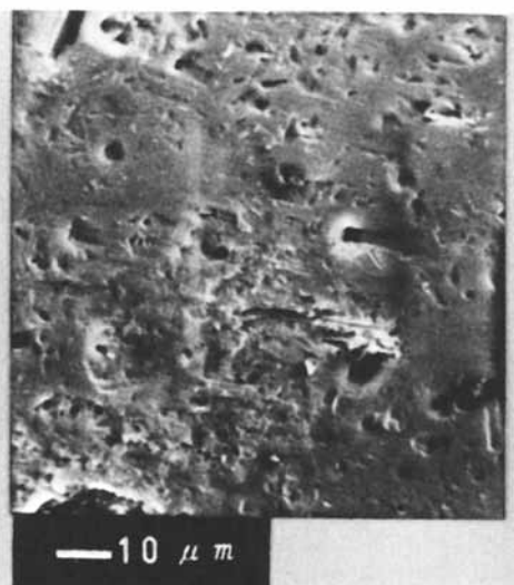
Figure 3. Surface structure of physically deteriorated membrane
