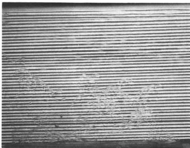
Figure 5. THF convection flow from the surface of polysulfone (15 wt % in THF). Elapsed time = 20 s.
