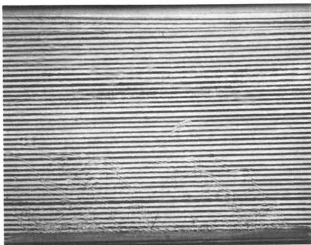
Figure 4. THF convection flow pattern in a water coagulating bath from cellulose acetate (20 wt % in THF). Elapsed time = 45 s.
