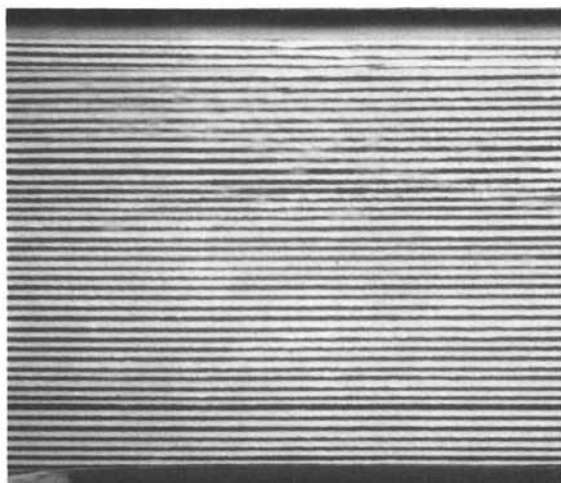
Figure 7. Coagulation of polysulfone (15 wt % in dioxane). Schlieren patterns were not detected. (This was the case for any coagulation of a polymer solution with a high specific gravity solvent.) Elapsed time = 45 s.
