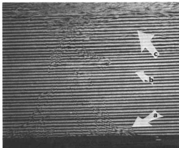
Figure 2. Detection of solvent (acetone) convection flows in a water coagulating bath; (a) surface of cellulose acetate (20 wt % in acetone); (b) acetone convection flow upward; (c) accumulation of acetone on the surface of the coagulation bath. Elapsed time = 45 s.
