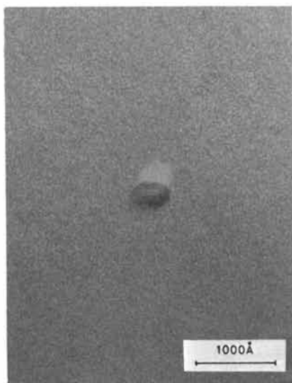
Figure 4. Electron micrograph of evaporated W particles. A carbon particle is shadowed ( \times 150,000 ).
