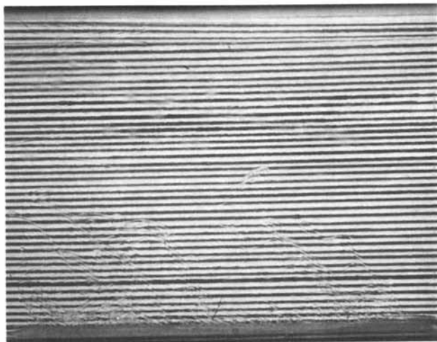
Figure 3. Acetone convection flows from the surface of cast cellulose acetate solution. Elapsed time = 10 s (see Table II).
